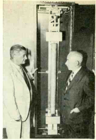
Rear section of Atomichron showing atomic beam tube. Left, Dr. Zacharias of MIT, key figure in the development; right, H. Guterman, board chairman of National Co.
